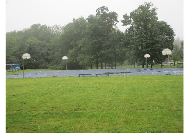
A rain garden can be installed south of the gazebo to capture, treat, and infiltrate rooftop runoff. Pervious pavement can be installed on the basketball court to store stormwater runoff and allow it to slowly infiltrate into the ground. A preliminary soil assessment suggests that more soil testing would be required before determining the soil's suitability for green infrastructure.
